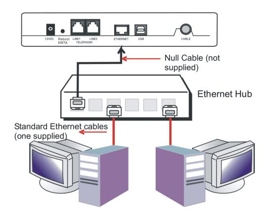
Fig.4: Ethernet Hub Connection
